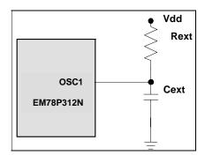
Fig. 5-33 External RC Oscillator Mode Circuit
